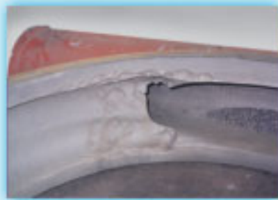
磨损的渣浆泵护套
