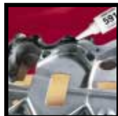
Loctite® 5910 Replacement for cork and paper cut gaskets on flanges and stamped sheet metal covers. Recommended for use where high vibration or flexing occurs. Can also be used with plastic and painted parts.
